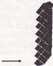
Figure 6: Effect of left to right screen printing on the edges of a vertical line.
