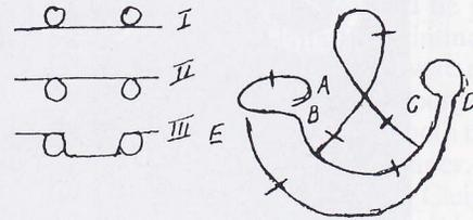
Figure 2. The concept of Mr. Loeber and Mr. van de Loo. The numbers I, II and III indicate the sequence of applying the metal thread, the turning over of the form, and the pounding out of the wire gauze of the form. The letters A, B, C, D and E follow the metal thread according to this concept. The cross hatches indicate the places where the thread is connected to the gauze of the form.
