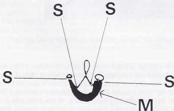
Figure 1. Dr. Reed's concept of the watermark. The body of the horn **M** is a solid plate of thin metal. The rest is metal wire, all soldered to the metal frame of the mold (form) **S**
