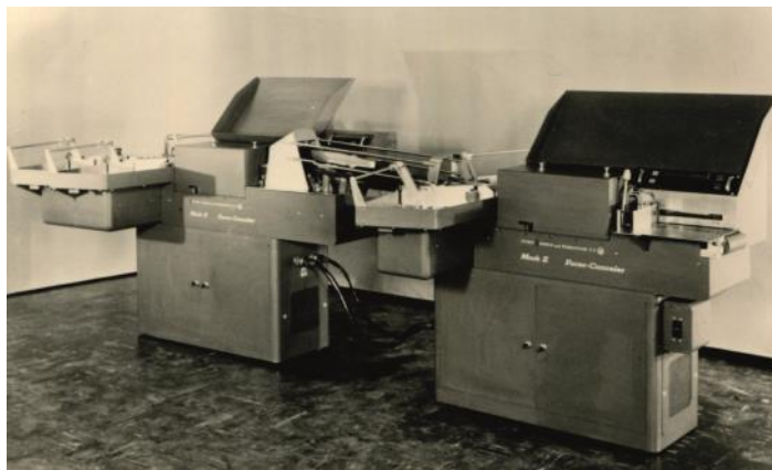
Figure 6: Tandem arrangement of two Mark II facers, allowing all mail to be faced and cancelled. Pitney Bowes, 1960.
