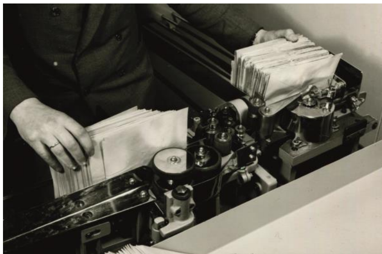
Figure 3: Photograph of machine-based postmarking of faced mail in the first half of the last century. All the covers are in the same – upside down - position, and with the address side facing the postal worker.
