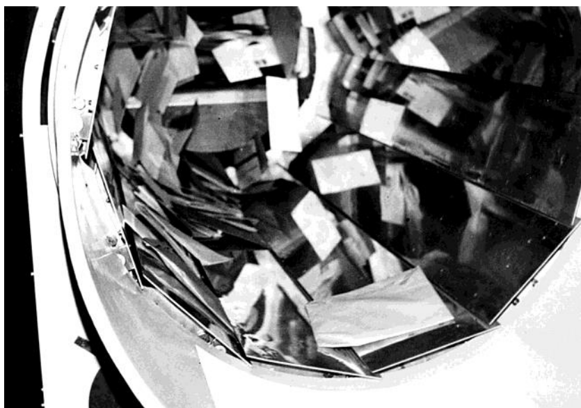
Figure 80: This photo, made by a member of the Study Group during an excursion, gives a glimpse into the inside of the culler. In the background we see the supply belt, delivering the mail items to the drum. The machine-suitable mail disappears through the slots in the wall on a conveyer belt, too thick mail is collected in a bin at the bottom of the drum and sent to manual processing.
