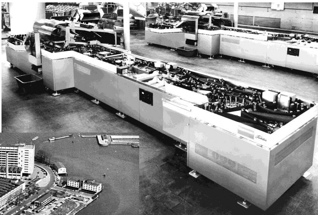
Figure 50: The two Toshiba culler-facer-cancelers that were installed and tested in August / September 1971 in the District Post Office in Amsterdam.
