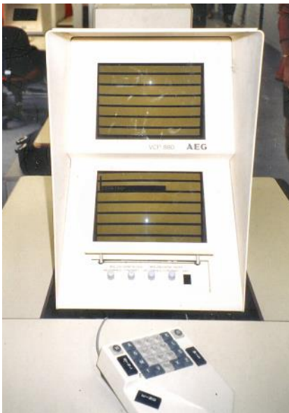
Figure 47: OVIS video coding station with the dual monitors and the keyboard.
