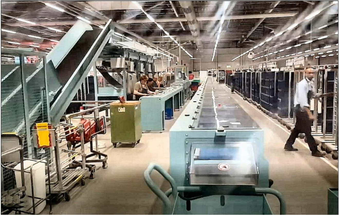
Figure 88: A sorting machine for the remaining mail with on the left side the conveyor belt on which the mail items are placed manually with the address side up. In the middle the sorting section.
