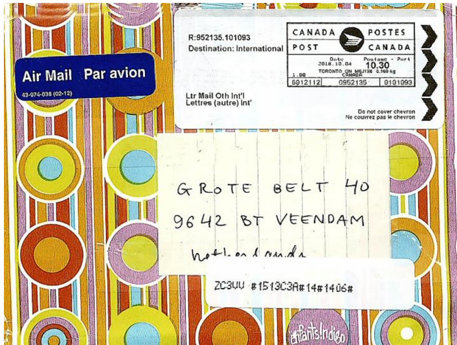
Figure 90: Mail item with a full sorting line PRIC applied by SMC number 3 in Sorting Center Zwolle. The PRIC has been applied to a white label. This PRIC type does not contain a postal code part.
