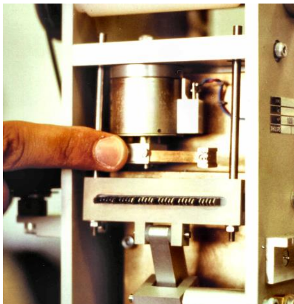
Figure 18: Part of a HIA sorting index printer from which the coding ribbon has been removed prior to taking the photo. Above the pins (a part of which was thrust forward during the rotating movement to 'write' the sorting index) is a hammer-mechanism on which a stamping device is mounted, which - also through the fluorescent ribbon - could apply a KPK imprint on the mail item. (Photo by author, taken in Rotterdam in 1982).
