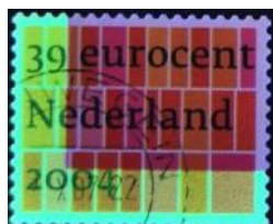
Figures 5a/b: Stamps with a vertical bar (left) or an L-shaped bar (right) that lights up green under UV illumination.
