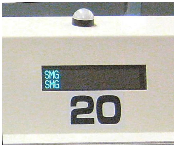
Figure 20: Mail pieces for further processing in a 'Sorteermachine-groot' (SMG) are collected in output stacker 20.
