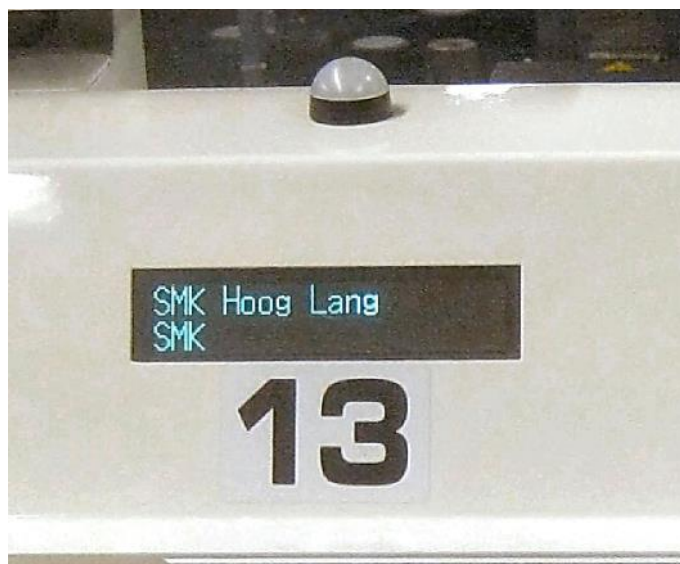
Figure 19: Mail pieces for further processing in a 'Sorteermachine-klein' (SMK) are collected in output stacker 13.
