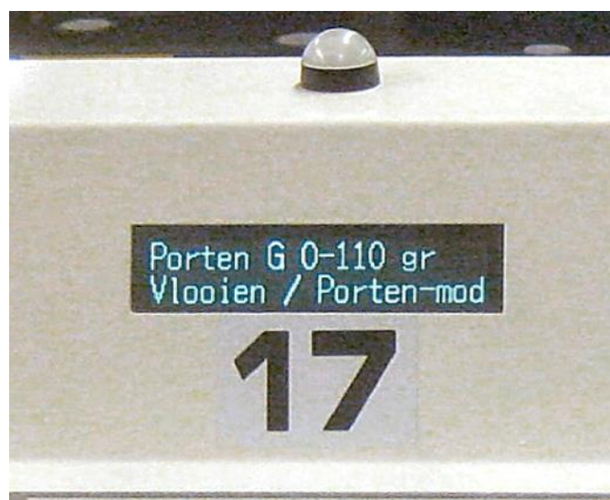
Figure 22: Output stacker 17 for postage taxable large-format mail items (character G = groot, large).
