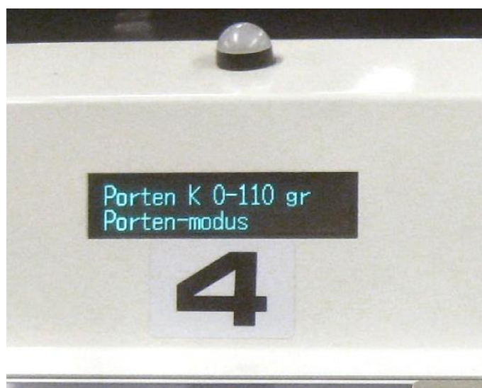
Figure 21: Output stacker 4 for postage taxable small-format mail items (character K = klein, small).
