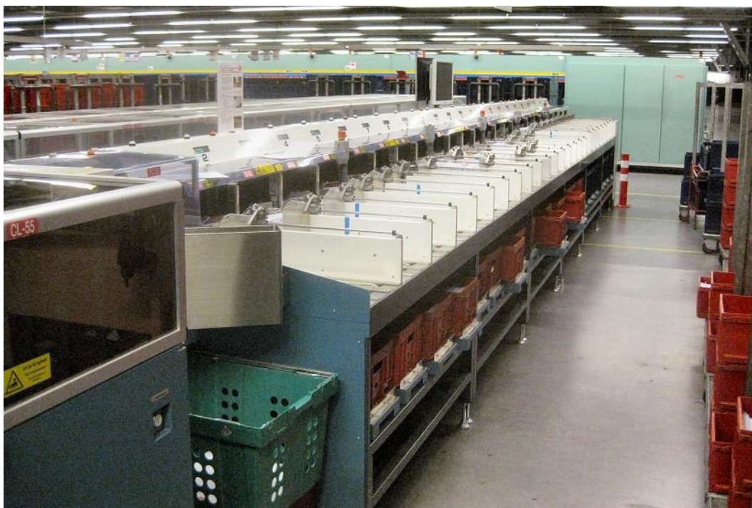
Figure 18: The 24 output stackers of an NEC NS-10 CFCs at Sorting Center Nieuwegein.
