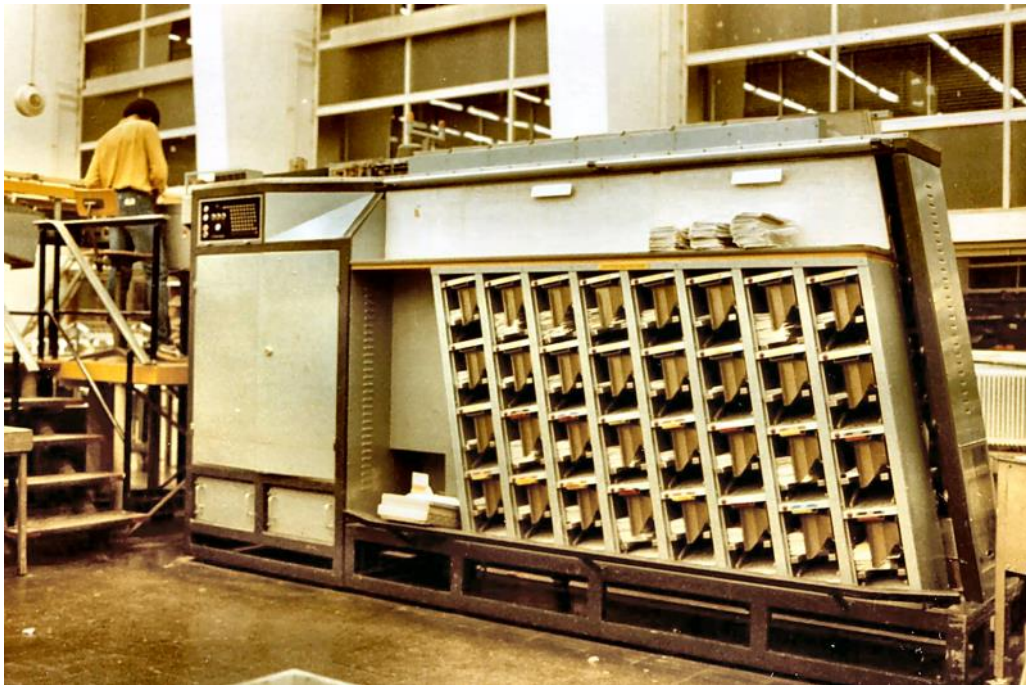
Figure 9: The sorting machine with a view of the 32 sorting compartments at the front (photo dated: 10-01-1980). The letters run across the top of the machine to above the appropriate sorting bin.
